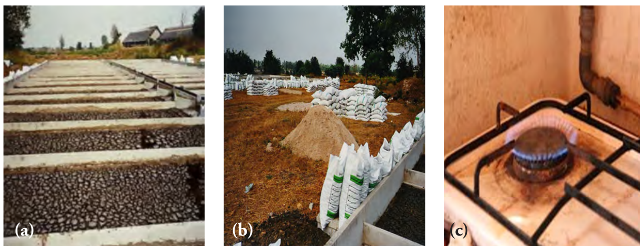
Figure 8: (a) Digestate from the biogas plant dried by the sun in ponds. (b) Packaged digestate to be collected by local farmers as fertilizer. (c) Biogas supply to village used for cooking gas that substitutes for the purchase of LPG
