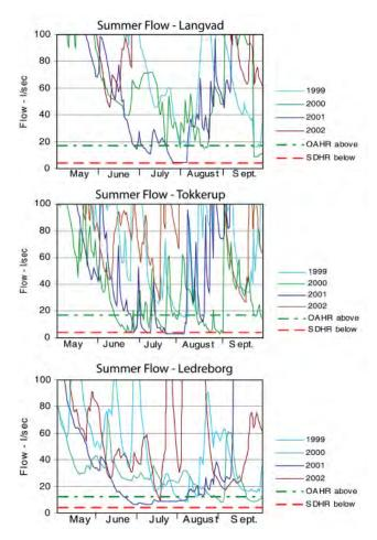
Figure 9. Hydrograph of the flows recoded over the summer months (May 1 – Sept. 30) for the three streams. The habitat limits for juvenile brown trout, as determined by the RHYHABSIM model, are shown. The flows that were above the OAHR line provided the optimal habitat area, where as the flows below the SDHR line were in the critical flow area. Note how in 2001 Langvad and Tokkerup reached SDHR limit for more than one week, where as Ledreborg remained above the SDHR limit during the same period.
