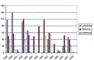
**Figure 8.** Bar graphs showing the number of days during the year that the stream flow dropped into the SDHR (top) and was below the OAHR (bottom).
