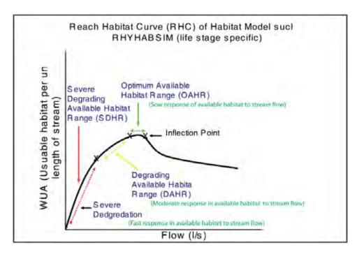
**Figure 5.** Diagram illustrating the different flow ranges (SDHR, DAHR and OAHR) as interpreted from a reach habitat curve.
